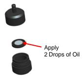
Figure 4-4: Apply 2 Drops of Oil to Impactor Plate
