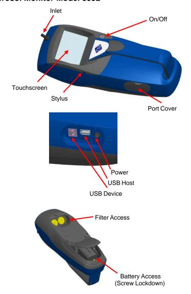
Figure 1-3: Features on Handheld Model
