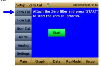
Run **Zero Cal** the first time the instrument is used and repeat prior to every use. Zero Cal requires that the zero filter be attached prior to running. Zero Cal must also be performed if the unit is reading negative concentrations. It is not possible for the DustTrak to read negative concentrations. Negative concentrations are a symptom of zero drift.
