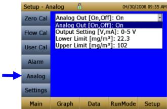
**Analog** setup screen sets the parameters that will drive the analog out port. Applies to the 8530 Desktop model only.
