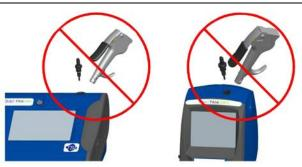
Figure 4-3: DO NOT Blow into Instrument
