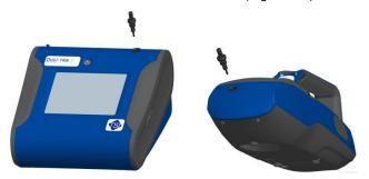
Figure 4-2: Unscrew Inlet Nozzle
